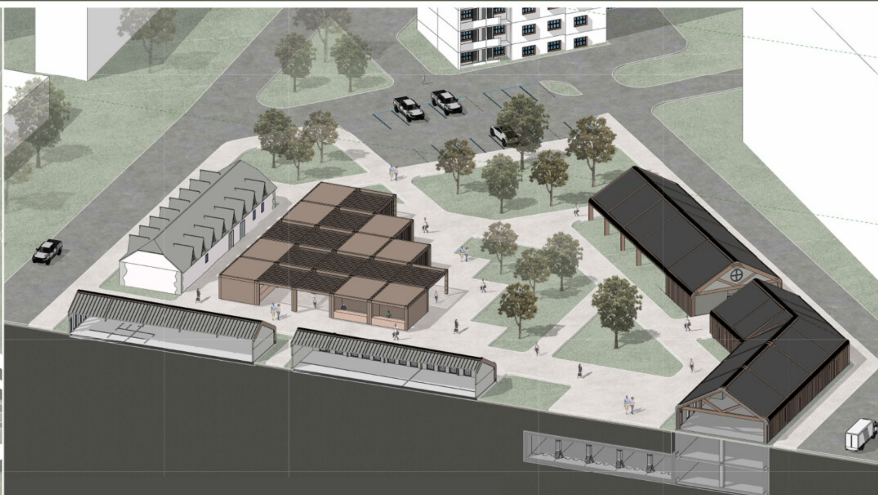
The designed market units integrate with the existing structure, featuring a planned square, semi-open modules for public sales, a social space supporting entrepreneurship, and an underground modular shelter.
